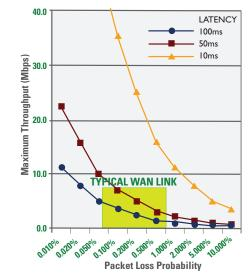
Bandwidth, latency, and loss have a significant impact on effective throughput across the WAN.
