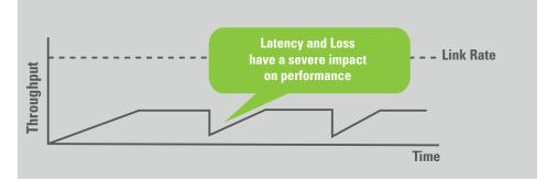
Periods of packet loss can have a "saw tooth" effect on WAN throughput, exacerbating the ill affects of latency.
