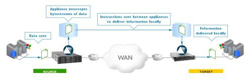
Network Memory uses real-time byte-level deduplication to eliminate the transfer of repetitive data across the WAN.
